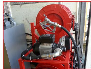
Thanks to the diesel tank placed in the maintenance vehicle, the work machines operating in the field of operation, excavation vehicles and all the equipment required for the supply of diesel supplies are provided without interruption. Tank capacity is determined according to customer preference and in-car settlement is considered. Alternative solutions are presented with diesel pumps and meters with different efficiencies determined according to work intensity.
